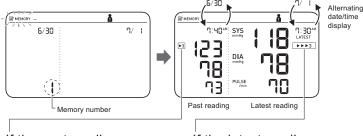
If the past reading was taken in TruRead mode, the "s" symbol appears and the reading shown on the left is the average of 3 measurements.
