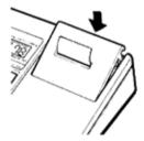
NOTE: The supplement ink roller should last about two years, however, if you need to replace the supplement ink roller, simply grasp the top of the ink roller and turn itslightlycounterc1ockwise before lifting the roller from the printer.
