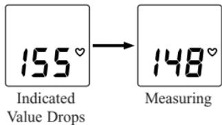
4. When the measurement is complete, the Heart Symbol (♥) stops flashing and your blood pressure and pulse rate are displayed alternately. Results will be displayed until you turn the unit off. The unit will automatically shut off in approximately 5 minutes.
