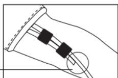
**NOTE:** Do not block the end of the short tube which contains a supplemental air release device that is necessary to maintain a proper deflation ratio. Blocking this tube may result in an inaccurate reading.
