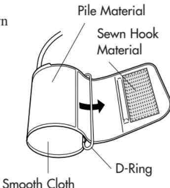
3. Put your left arm through the cuff loop. The bottom of the cuff should be approximately 1/2 inch above the elbow. The green marker on the cuff should lie over the brachial artery on the inside of the arm. The cuff tube should run down center of arm even with middle finger.
