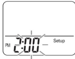
**4. Press the MEMO/▲ Button to advance by increments of one minute.**
