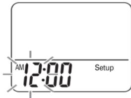
**2. Press the MEMO/▲ Button to advance by increments of one hour.**
