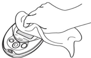
**Do not immerse the unit or any of the components in water.** The unit is not waterproof. Do not wash it or touch it with wet hands. Be careful that water does not get into the unit.
